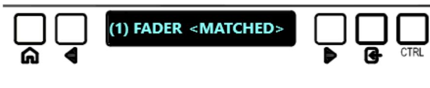
The fader position now matches the Recall store. The auto scan process will continue until it discovers another pot or fader position out of place from the saved console store.
