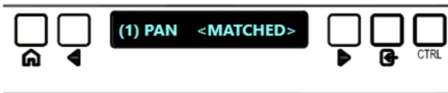
The pot position now matches the console store. The auto scan process will continue until it discovers another pot or fader position out of place from the saved Recall store.
